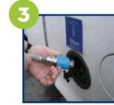
Retract the sleeve on the nozzle and push connector onto receptacle
