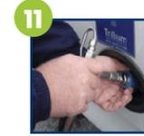
Pull back on the sleeve to remove the nozzle
