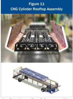
IV cylinders are the lightest in weight, being made of a polymer liner fully wrapped in a reinforcing composite.
